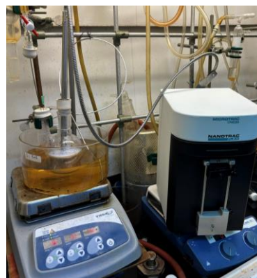
Fig. 1: Inserting Probe in Polymerization Reaction
